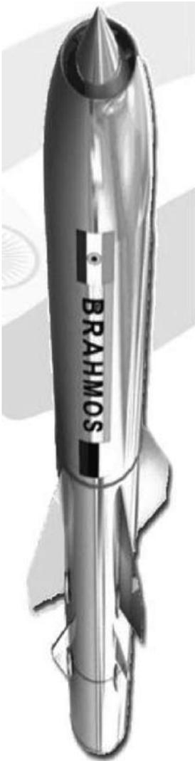
BRAHMOS is a two-stage missile with a solid propellant booster engine as its first stage which brings it to supersonic speed and then gets separated. The liquid ramjet or the second stage then takes the missile closer to 3 Mach speed in cruise phase. Stealth technology and guidance system with advanced embedded software provides the missile with special features.
