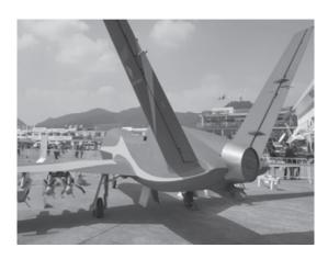
UAV's stealthy features include a jet engine hidden from enemy radar by a serpentine air intake, serrated panel edges, canted vertical stabilisers, as well as a faceted nose (Plate 2).<sup>11</sup> Its six hardpoints can carry a combined payload of 400 kilogram, including a wide range
